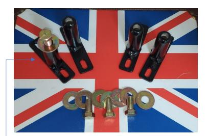
Step 1: Locate and Remove trim above 4 corner install positions. If installed; Remove stock rubber/aluminum rails, add ½ hole if needed to allow stock plastic trim to slide over provided Stantions. **TIP:** Install rack and center, tighten roof hardware, remove rack, then hold corresponding roof trim over stantion, drill hole in trim. NOTE: **CURVED** STANTION GOES IN FRONT OF RACK
